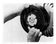
Figure 2.9 Removing a Taper Lock® bush
