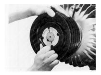
Tighten screws alternately Figure 2.7
